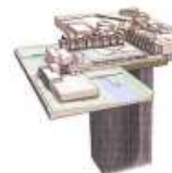
Vertical heat exchanger fields 50 to 200 m deep
